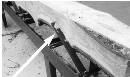
Place flat side, flush against squaring pin to ensure a square cant.
