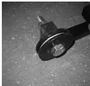
Track wheel, keep groove clean and lightly oiled.
