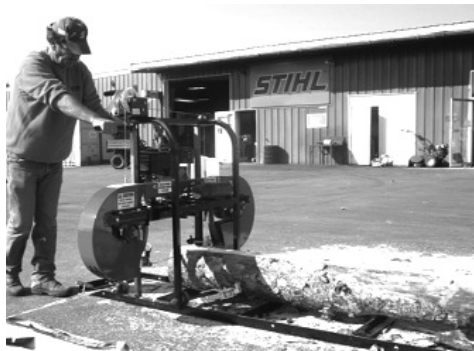
#3. Adjust blade height, rev engine.
