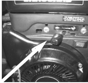
Engine throttle lever, always run engine full throttle when cutting.
