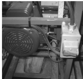
Electric mill, 220 volts, on/off switch.
