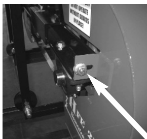
Remove guard nuts to remove blade guards to change blade.
