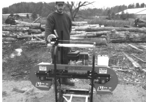
Correct head placement; Operators side is on side with the scale stick.
