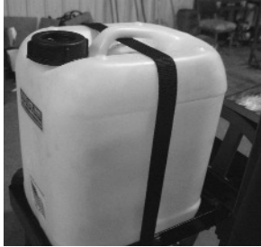
Lube tank for blade lube.
