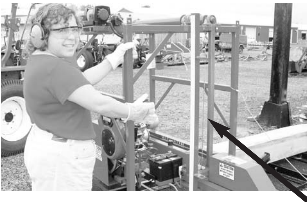
Correct head placement; Operators side is on side with the scale stick.
