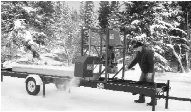
Correct trailer set up - All legs are level; head should not move on its own.
