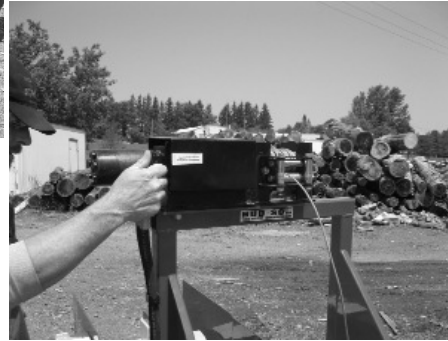
8.) Push in winch lever to disengage winch, turn until it is locked against plate.
