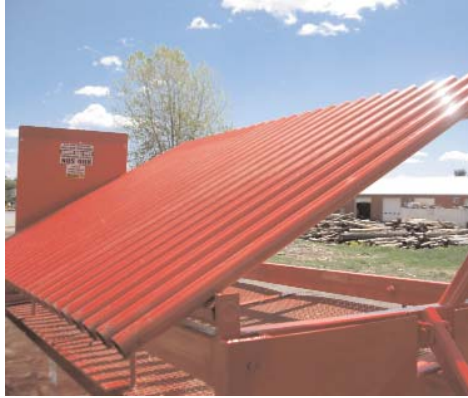
Grizley bars, keep clean during use. Use bucket to flip up and dump trash on ground.
