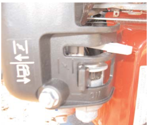
Engine choke and fuel shut off. Turn off fuel before transporting on highway.
