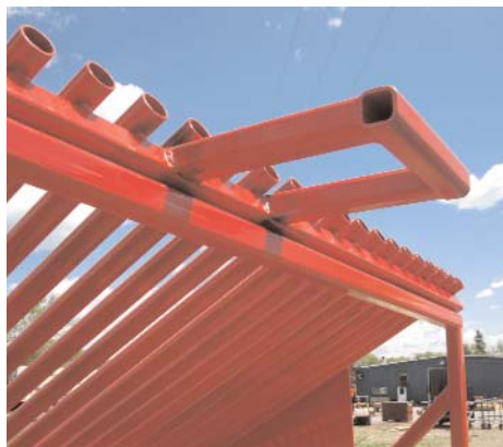
Grizley bar lifting horn, check daily for cracks or damage on all Grizley bars and horn.
