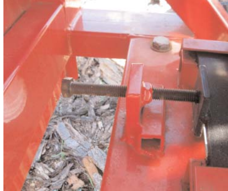
Belt tensioner bolt, keep lubed to prevent rusting. To tighten belt screw in belt tensioner bolt. Do NOT over tighten. Belt should have 1/4" to 1/2" free play at center of belt.
