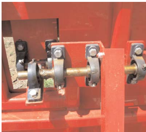
Shaker assembly bearings, lube daily (two shots of grease per bearing).
