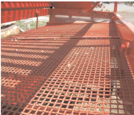
Dirt screen, clean out small stones that may wedge in screen daily or as needed during use.
