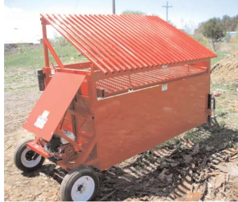
Spoil side of Screener, all waste material comes off this side.
