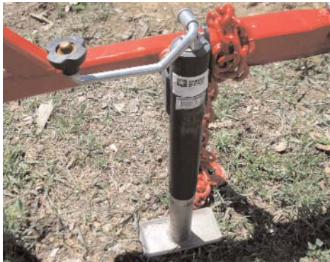
Set screener level using jack and side legs.
