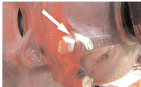
Gear reduction box oil level check plug, machine must be level when gear box oil level.
