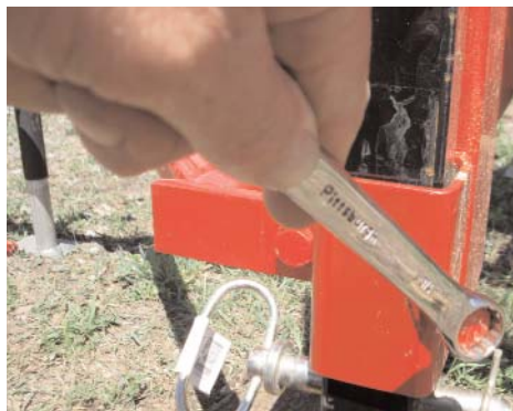
Tighten set bolt after screener weight is on legs.
