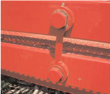
Loading side Dog Bone, grease daily. During heavy use, grease every 3-4 hours.
