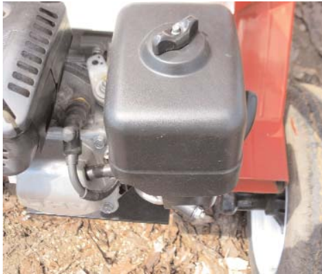
Air filter, clean daily, in dusty conditions clean every 3 to 4 hours.
