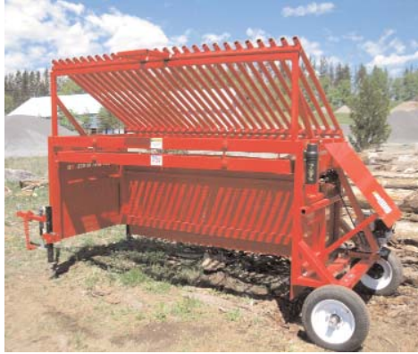
8-M Screener loading side and screened material removal side.
