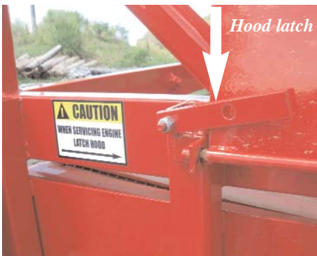
Engine hood in raised position. Be sure to latch hood in raised position when servicing engine and machine.
