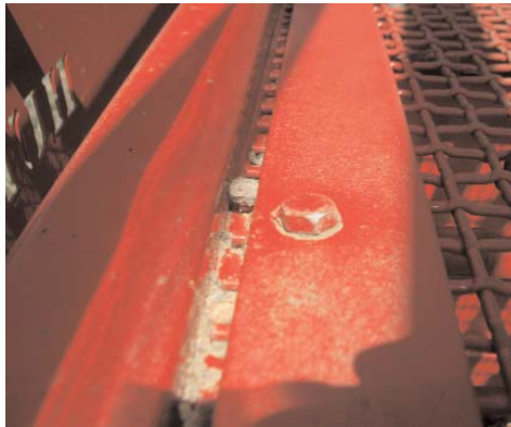
Screen retainer plate. One at each end and one in the middle. Check before operation each day for broken or missing bolts.
