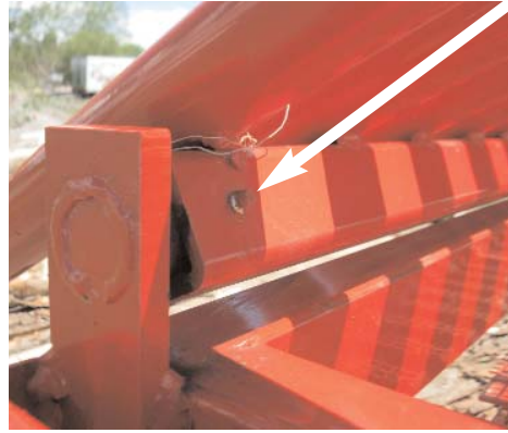
Grizley rack swivel point. Grease at both ends twice weekly.
