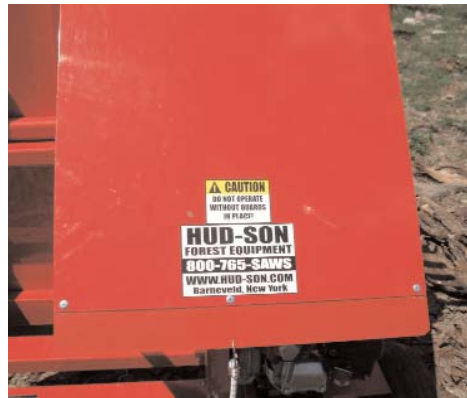
Engine hood in down position, keep down during operation.
