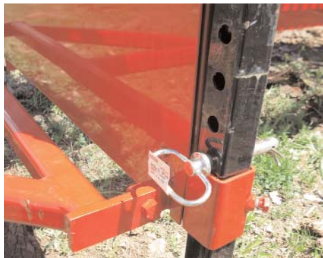
After leveling with jack set leg pin to bottom of leg holder to adjusted height needed.
