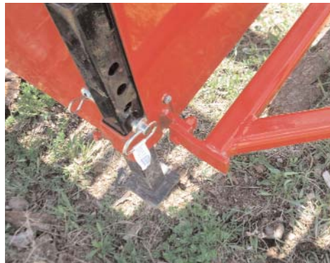
Use leg pins to keep screener from settling.
