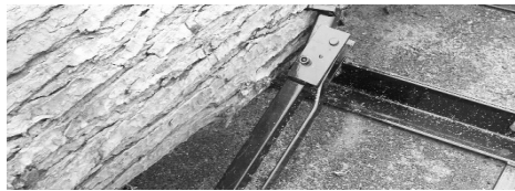
Adjustable dog, set at an angle so that the log can be sawed without interference.
