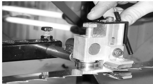
Pictured is a close-up of the guide It shows all the bolts and bearings that can possibly be adjusted. Note how the teeth are outside of the guide.
