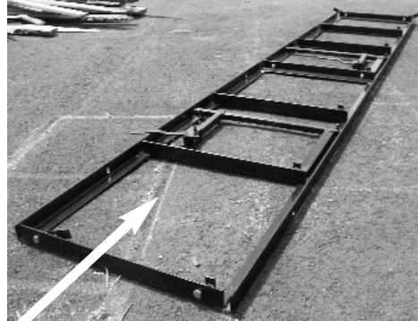
Squaring arm on right, adjustable dog on left.
