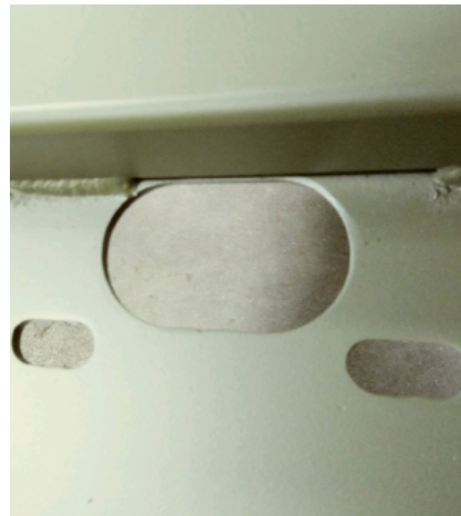
Engine oil drain hole in the motor mount plate.
