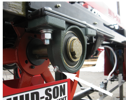
Pillow block bearings. Grease every 80 hours of use
