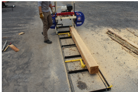
#5. Cut log into desired dimensional lumber.
