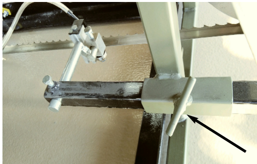
Adjustable blade guide bar and T handle locking bolt.
