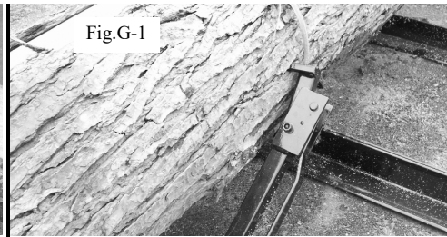
Adjustable dog, set at an angle so that log can be sawed without interference.
