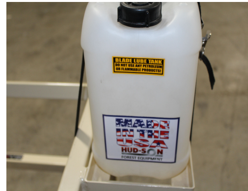
Blade lube tank, keep adding during use and be sure to drain in cold weather.
