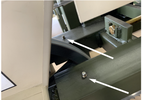
Tension wheel slide plates. Grease as needed both sides of head.
