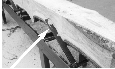
Place flat side, flush against squaring pin to ensure a square cant.
