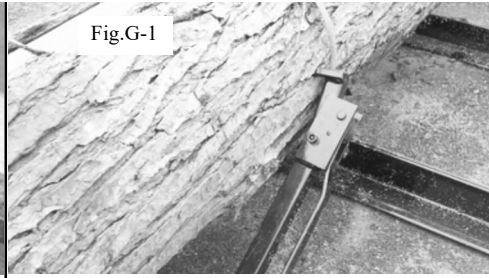
Adjustable dog, set at an angle so that log can be sawed without interference.
