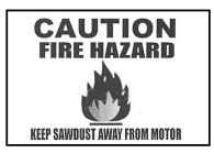
Check the engine compartment for sawdust and wood trash build up in and around the engine compartment and the exhaust area to prevent any possible fires from starting due to excessive build up. Always clean the sawdust out from under the machine after shut down and be sure there is no sawdust build up near or around the muffler area.
