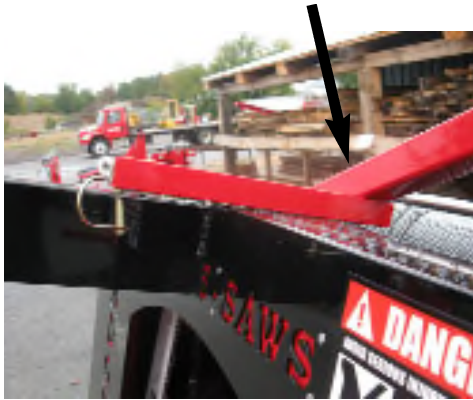
Saw bar arm shown in locked position for road travel
