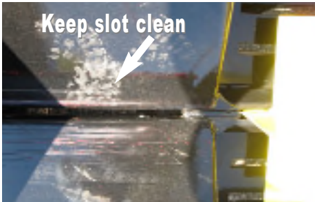
Splitter tray, keep this area clear of debris
