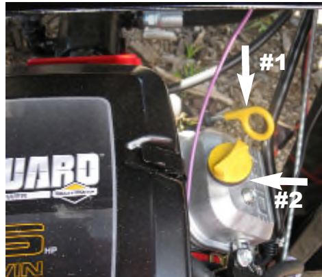
#1: Engine oil check stick; #2 Engine oil fillport
