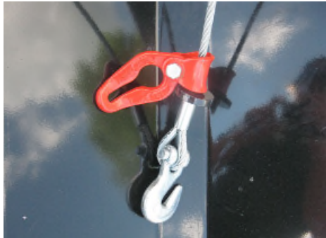
Keyhole slide chain grab grab hook on end of winch cable
