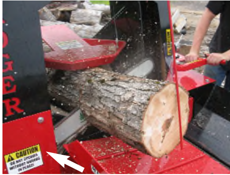
Bar maintenance guard
