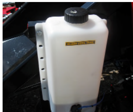
Bar oil tank
