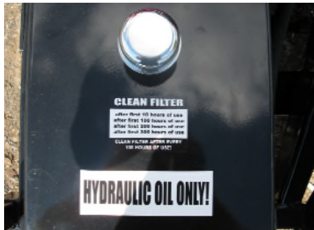
Hydraulic oil tank vent cap and fill port
