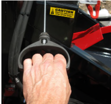
Log hold down handle oil pulley and cable
