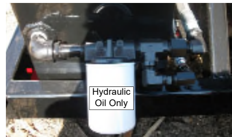
Hydraulic oil filter - takes AW-32-WT hydraulic oil. Replacement 40-20 Hyd filter
