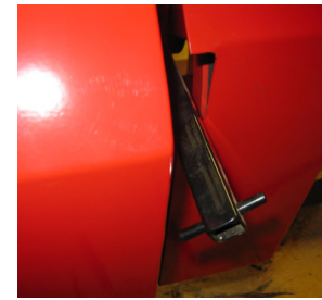
Part #24 - extended guard fastener to remove guard for blade change.
