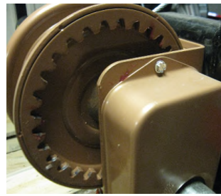
Use a light grease for winch sprocket.
