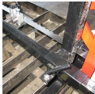
Adjustable blade guide bar and locking bolt.
