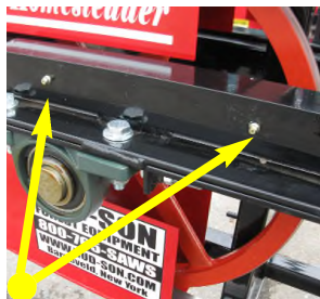
Tension wheel slide plates. Grease as needed both side of head.
