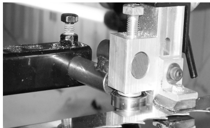
Pictured is a close-up of the guide. It shows all the bolts and bearings that can possibly be adjusted. Note how the teeth are outside of the guide.
