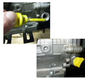
Engine oil check and fill port
