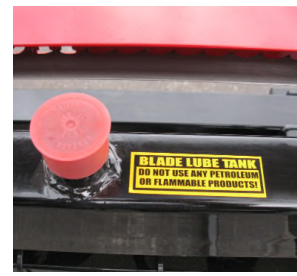
Blade lube tank, keep adding during use and be sure to drain in cold weather.
