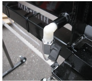
Blade lube flow valve on/off adjustable flow.
