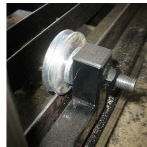
Keep groove clean - track wheel, light oil
