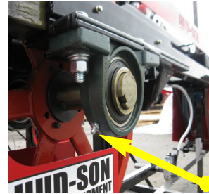
Pillow block bearings. Grease weekly.
