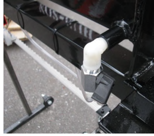
Blade lube shut of valve
