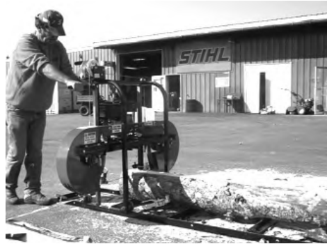
#3. Adjust blade height, rev engine.
