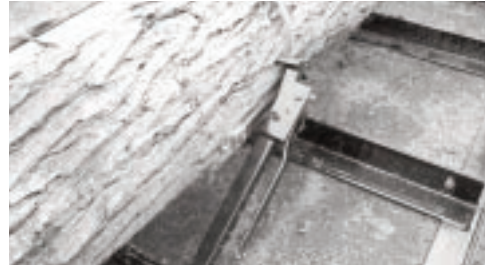
Adjustable dog, set at an angle so that log can be sawed without interference.
