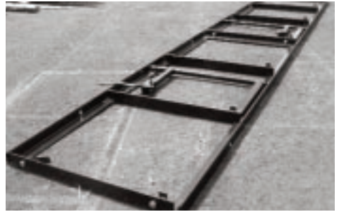
Squaring arm on right, adjustable dog on left.
